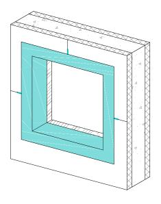
APPLY DYMONIC 100 3" MIN INTO ROUGH OPENING AND EXTERIOR FACE OF WALL AT SILL, JAMBS, HEAD
