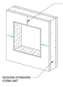
VERTICAL AND HORIZONTAL SEAMS MUST BE DETAILED WITH DYMONIC 100 FROM EDGE OF OPENING AND EXTEND BEYOND FLASHING MATERIALS BY 1" MINIMUM; VERTICAL SEAMS REQUIRE THE DYMONIC 100 TO GO BACK TO CONCRETE FACE AND FILL VERTICAL SEAM
