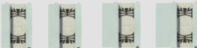
1" (25mm) R-value - 28 U-value - 0.21 2" (50mm) R-value - 32 U-value - 0.18 4" (100mm) R-value - 40 U-value - 0.15 6" (150mm) R-value - 48 U-value - 0.12
