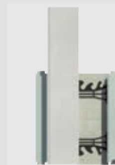
6" (150 mm) concrete core R-Value ratings based on exterior brick finish
