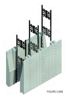
With T Forms, the main wall exterior panel is also molded from a common sized mold that is intended to be adapted for ALL core thicknesses of T Form. For this reason, remember that the main wall panel will require component assembly and form support on site for 4, 8, 10 and 12-inch (102,203,254 and 305 mm) core forms.
