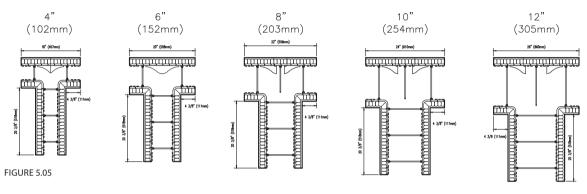
For Double Sided Tapered Top Forms and Double Sided Brick Ledge Forms, the products will arrive to site shipped with separate standard panels. This is because the same molds that are used for forming standard assembled tapered top and one side brick ledge forms are used for these products as well with fastening strips installed instead of fully assembled hinge pin webs. Be sure you accommodate for these nuances on your product counts and quantities.
