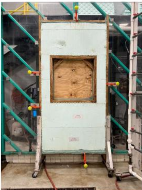
Diagram 1: 8' x 4' (2.4 m x 1.2 m) Nudura Prebuck Assembly
