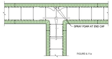
Nudura also recommends bracing the T Wall forms internally by using the following method; Place horizontal reinforcement within the main wall, extending one or two webs past each side of the T connection (See "Position A", Figure 6.11a) then cut two pieces of reinforcing steel 1" (25 mm) longer than the cavity width, inserting at either the first or second web (See "Position B", Figure 6.11b) in the T connection and tie to the reinforcing steel in the main wall.
