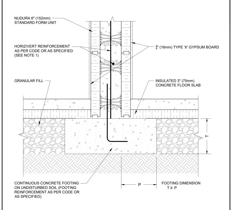
1) FOR OPTIMAL REINFORCEMENT PLACEMENT IN THE NUDURA FORM, SPACING OF HORIZONTAL REINFORCEMENT TO BE SPECIFIED AT 18" (457mm) O.C. AND VERTICAL REINFORCEMENT TO BE SPECIFIED AT MULTIPLES OF 8" (203mm) O.C. REFER TO NUDURA REINFORCEMENT PLACEMENT DETAILS.
