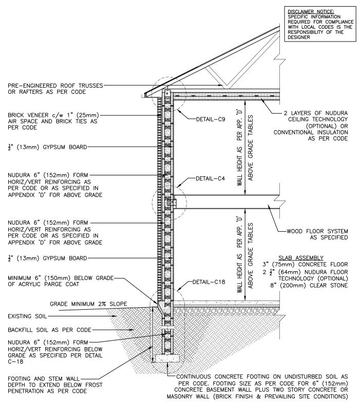
\*NOTE: IN ADDITION TO FOOTING SIZE INDICATED BY CODE, ADD 1" (25.4mm) WIDTH TO STRIP FOOTING FOR EVERY 1'-0" (305mm) OF CONCRETE WALL HEIGHT ABOVE 8'-0" (2440mm) PER STORY
