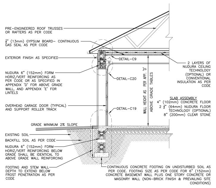
\*NOTE: IN ADDITION TO FOOTING SIZE INDICATED BY CODE, ADD 1" (25.4mm) WIDTH TO STRIP FOOTING FOR EVERY 1'-0" (305mm) OF CONCRETE WALL HEIGHT ABOVE 8'-0" (2440mm) PER STORY
