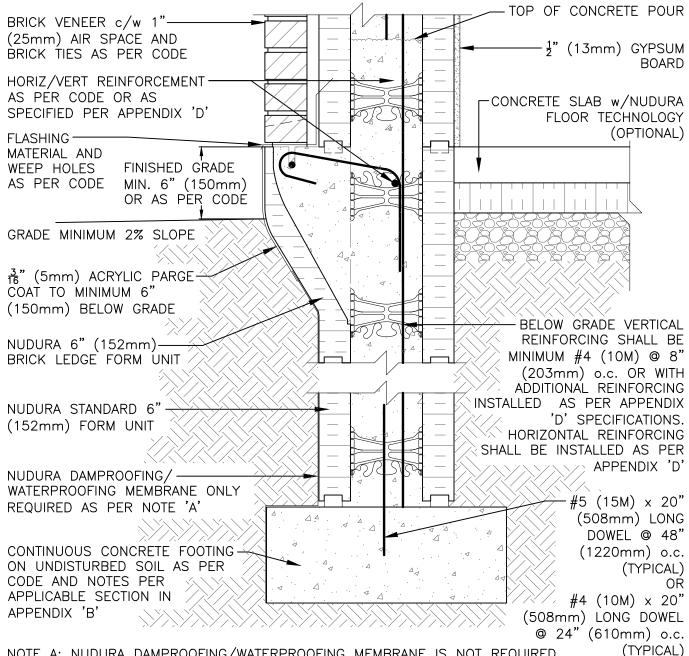
NOTE A: NUDURA DAMPROOFING/WATERPROOFING MEMBRANE IS <u>NOT</u> REQUIRED EXCEPT WHEN THE INTERIOR FINISHED FLOOR LEVEL IS BELOW THE EXTERIOR FINISHED GRADE LEVEL
