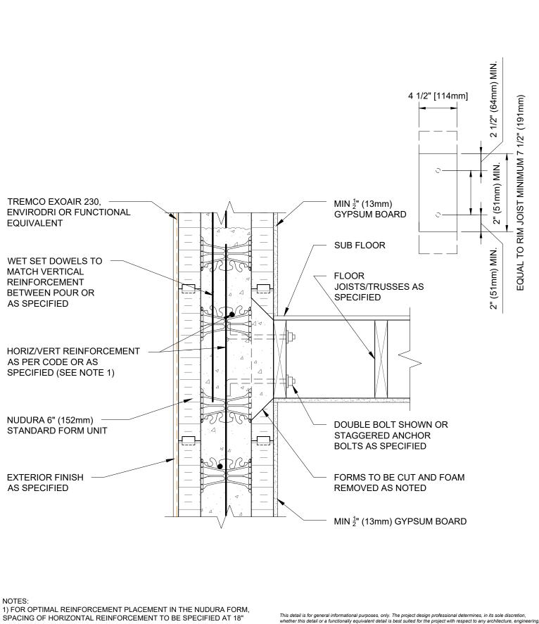
(457mm) O.C. AND VERTICAL REINFORCEMENT TO BE SPECIFIED AT MULTIPLES OF 8" (203mm) O.C. REFER TO NUDURA REINFORCEMENT PLACEMENT DETAILS.
