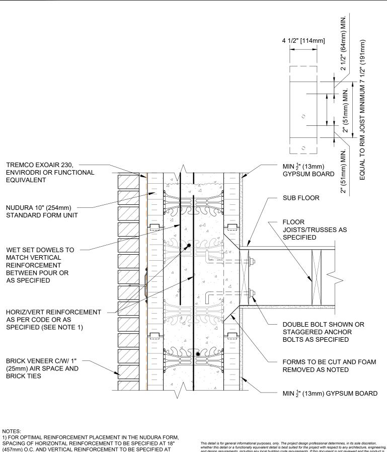
MULTIPLES OF 8" (203mm) O.C. REFER TO NUDURA REINFORCEMENT PLACEMENT DETAILS.
