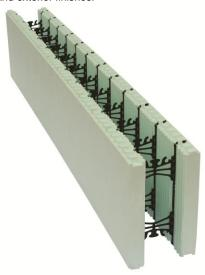
Both the EPS panels and web/fastening strips are molded with a preformed reversible interlock and vertical clip-locking mechanism on their top and bottom edges to facilitate stacking and vertical inter-locking of the form units.
